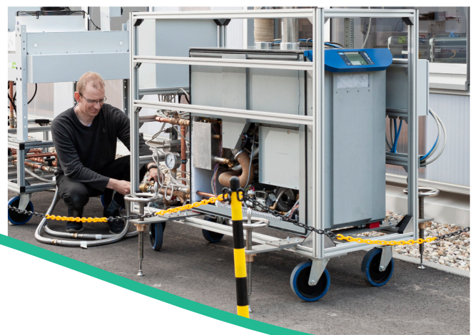
Micro gas turbine testing operations: Installation of water mass flow sensors
