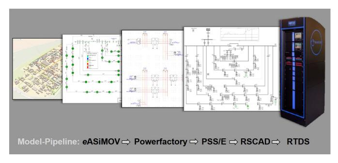
An example of the EGSAL modeling pipeline showing the KIT 20kV campus north network from the model in the eASiMOV framework to the converted model in the RSCAD software for real-time simulation.
